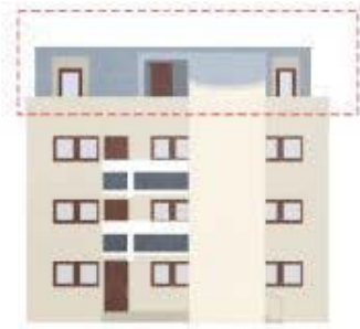
Roof extension provide additional dwelling(s) upstairs
