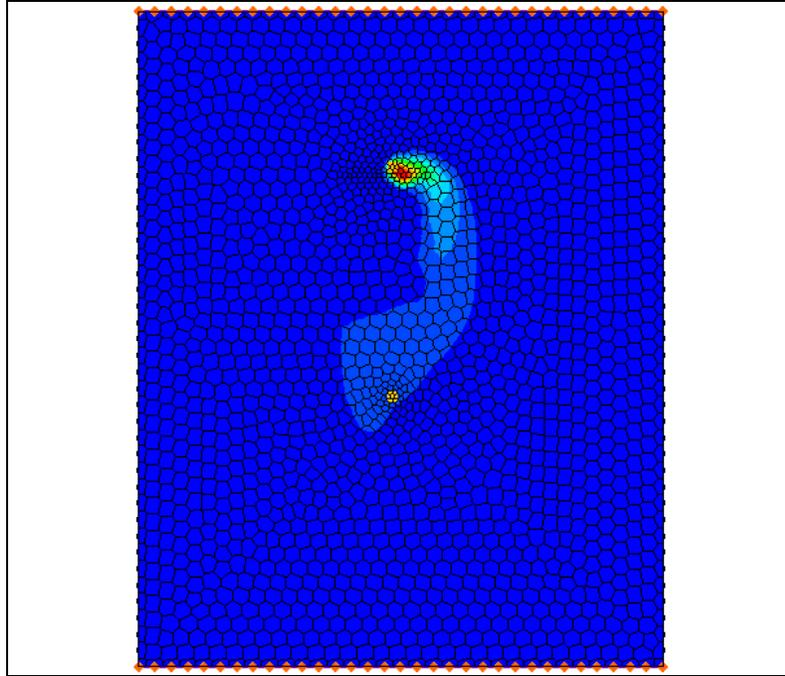
Figure 10 MODFLOW-USG Transport model using a voronoi UGrid
