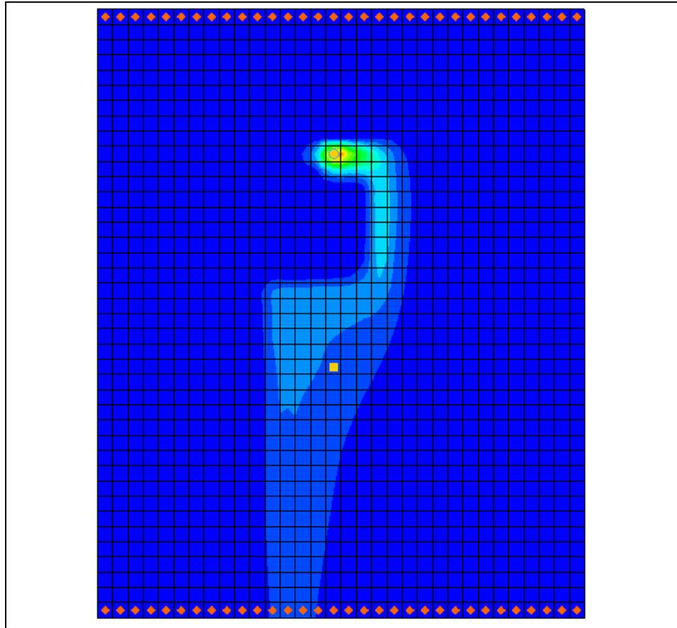
Figure 9 Contaminant plume from the MODFLOW USG-Transport solution
