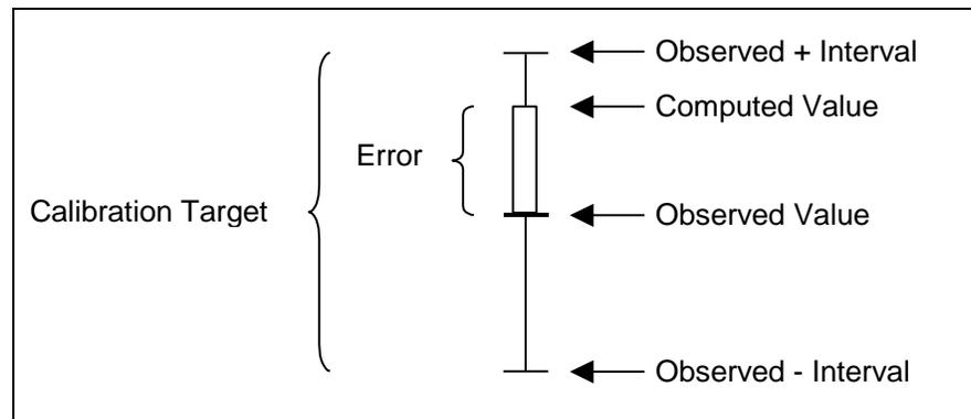
Figure 6 Calibration target
