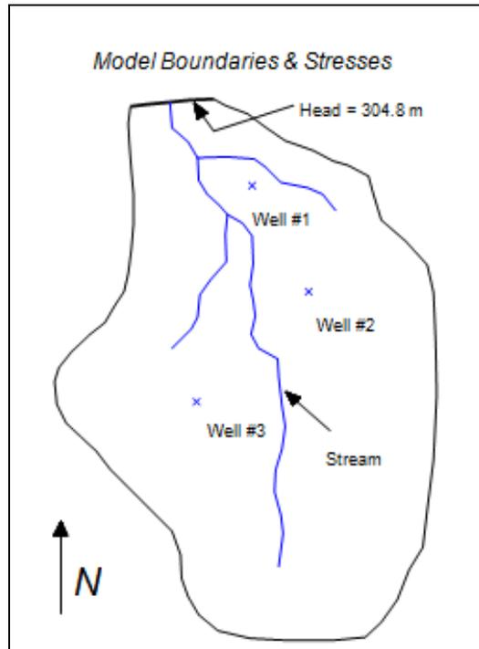
Figure 1 Sample model used in calibration exercise
