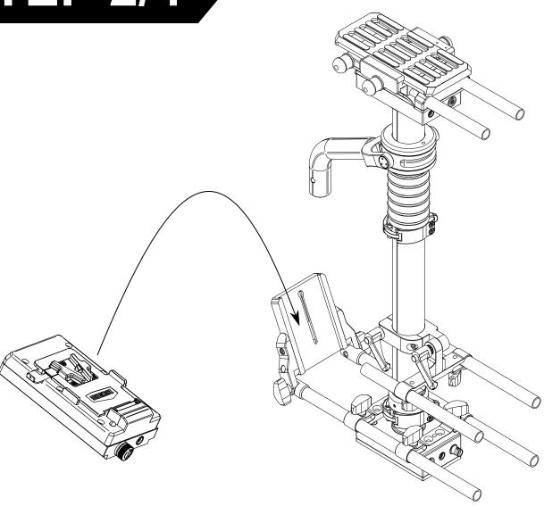
Slide into the universal battery adapter, the Vlock plate module and fix it to the adapter using one or two Photo Screws (1/4"-20 UNC ) in bundle with your kit.
