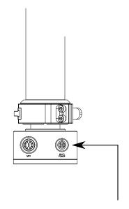
Connect the Battery module to the sled (MULTI POWER INPUT) using the specific cable (2 pin to 4 pin cable)
