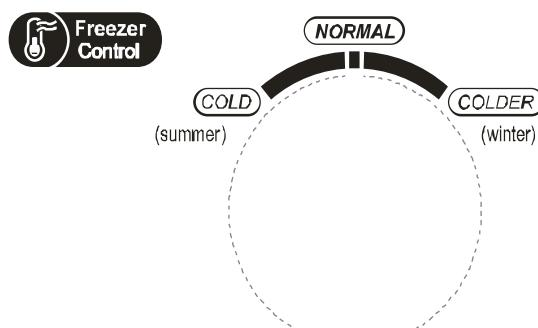
The freezing temperature is relatively low in "COLDER" position, while the freezing temperature is relatively high in "COLD" position, thus, "NORMAL" position is generally used.
