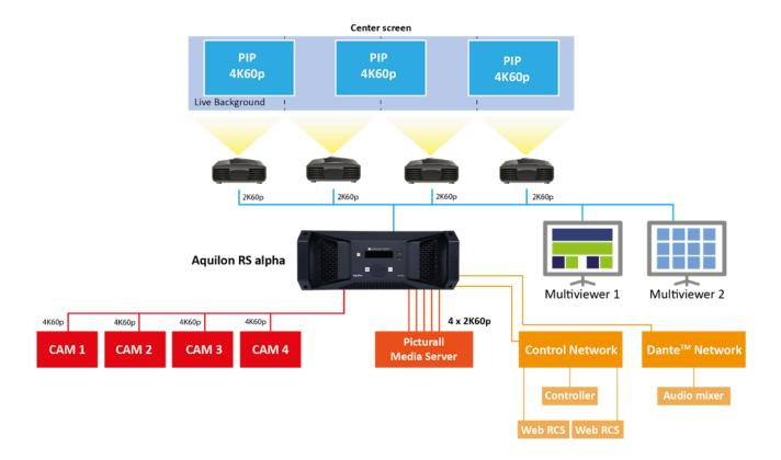
Aquilon RS alpha can drive one 8K60p LED wall with up to four 4K PIPs
