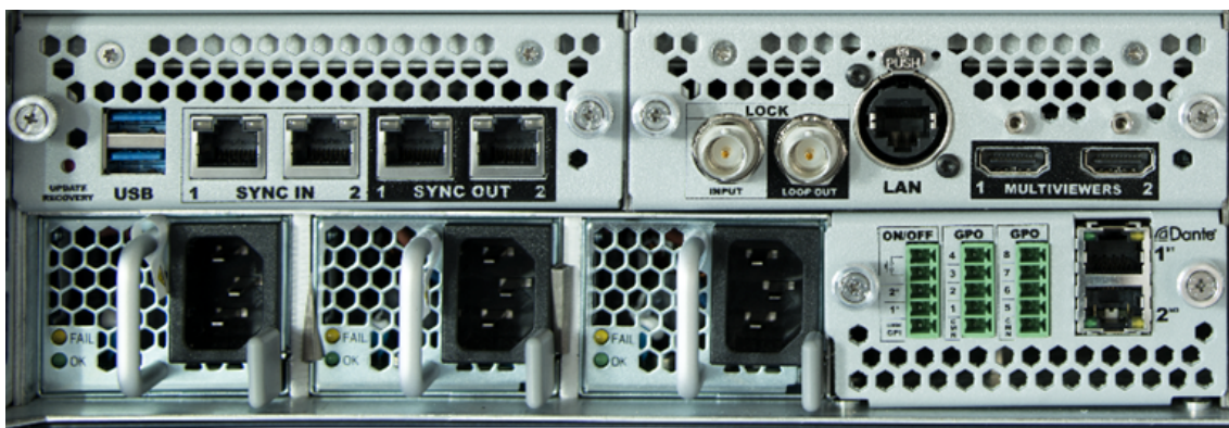
Fixed parts on all Aquilon units
