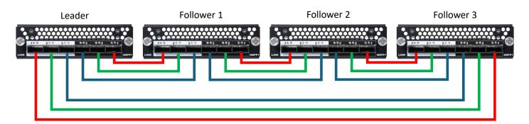
**IMPORTANT:** Please carefully respect the numbering of the connector (OUT 1 to IN1, OUT 2 to IN 2 and OUT 3 to IN 3)
